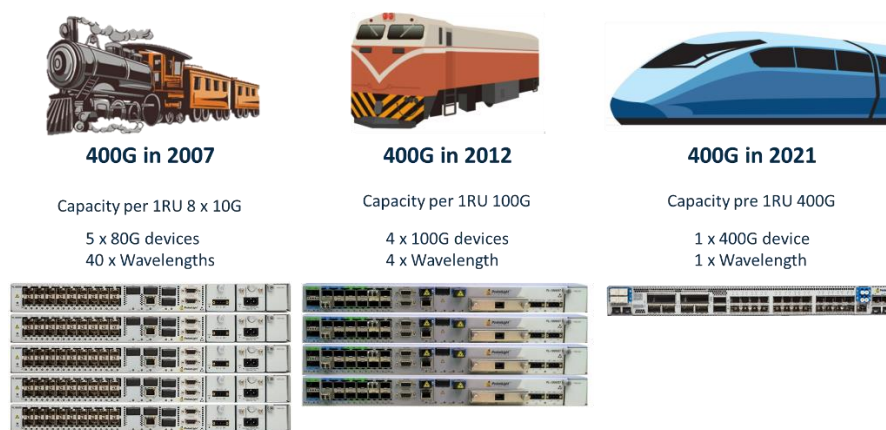
Figure 1: The evolution of 400G transport - from 40 wavelengths to four and now, one
